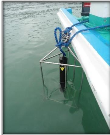
**Figura 18:** Correntómetro ADCP (Acoustic Doppler Current Profilers)
