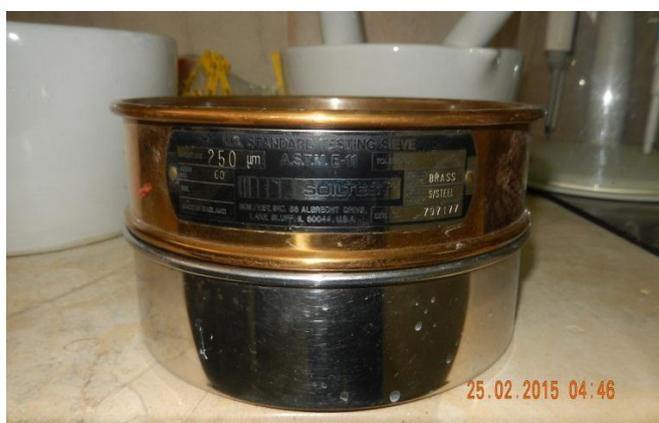
Figura 13. Tamiz (ASTM-A 11)
